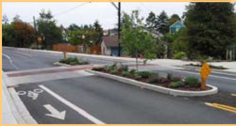
Mid-block crossing, raised with medians
