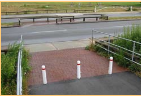
Mid-block crossing, offset at median
